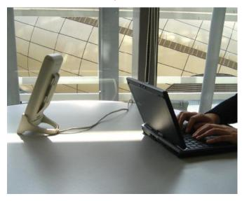
The Altai C1n employs patented smart signal processing algorithms and antenna design to increase WiFi signal strength (transmit and receive) by as much as 16 dB in areas covered by an A8n Super WiFi Base Station or A2 WiFi Access Point. It can be installed exactly where the throughput is required to boost up, and it allows the service operator to increase the coverage range of an A8n base station substantially and provides greater flexibility and cost savings to WiFi deployments.
